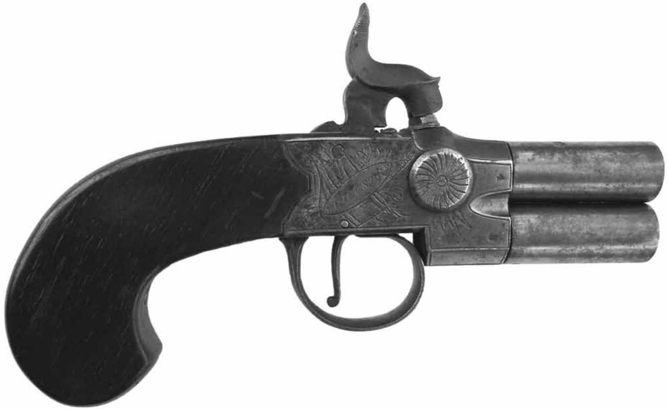
The pistol is of normal box lock construction, with a slab sided butt and two barrels in an over and under configuration. The barrels of about .36 calibre, are 1 ½ inches long and are smooth bored. The eight deep grooves filed into the muzzles of the barrels are for a key which is needed for their removal when loading.
