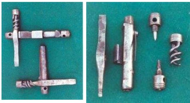
*Sergeant's combination tool dismantled showing, large and small blade screwdriver, pointed piercer and screw for drawing jammed bullets and double worm for cleaning. The body incorporates a nipple key and pricker with a main spring clamp on the side, and internally is an oil bottle.*
